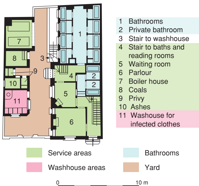
Plan of the country's first public wash house, built in Liverpool in 1842, showing an internal layout that may have been similar to that in the Manchester Baths and Wash House
