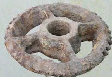
A bevel gear from the 1792-3 power system
